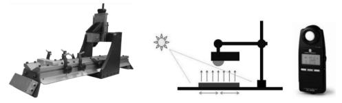
Figure 2: MOR test device (left) and colour test device (right)
